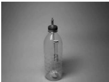
Figure 2. Plastic bottle with a test tube covered by a rubber membrane.
