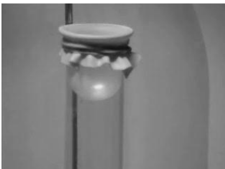
Figure 2. Plastic bottle with a test tube covered by a rubber membrane.
